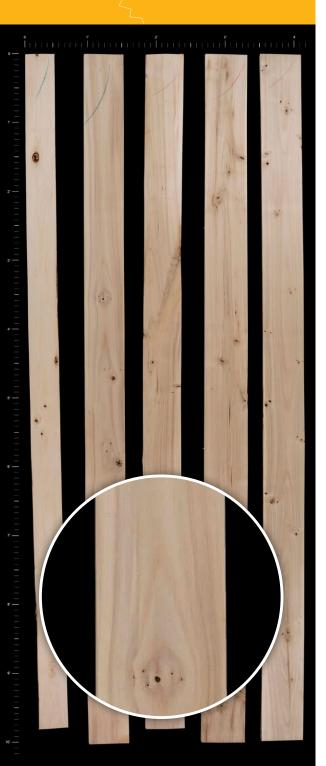
Cottonwood Chop grade boards provide structural grade boards for upholstery frame construction and crating.
